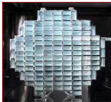
This aerogel array, which was mounted atop the Stardust spacecraft, was used to collect interstellar dust particles as well as dust from the tail of comet Wild 2.
